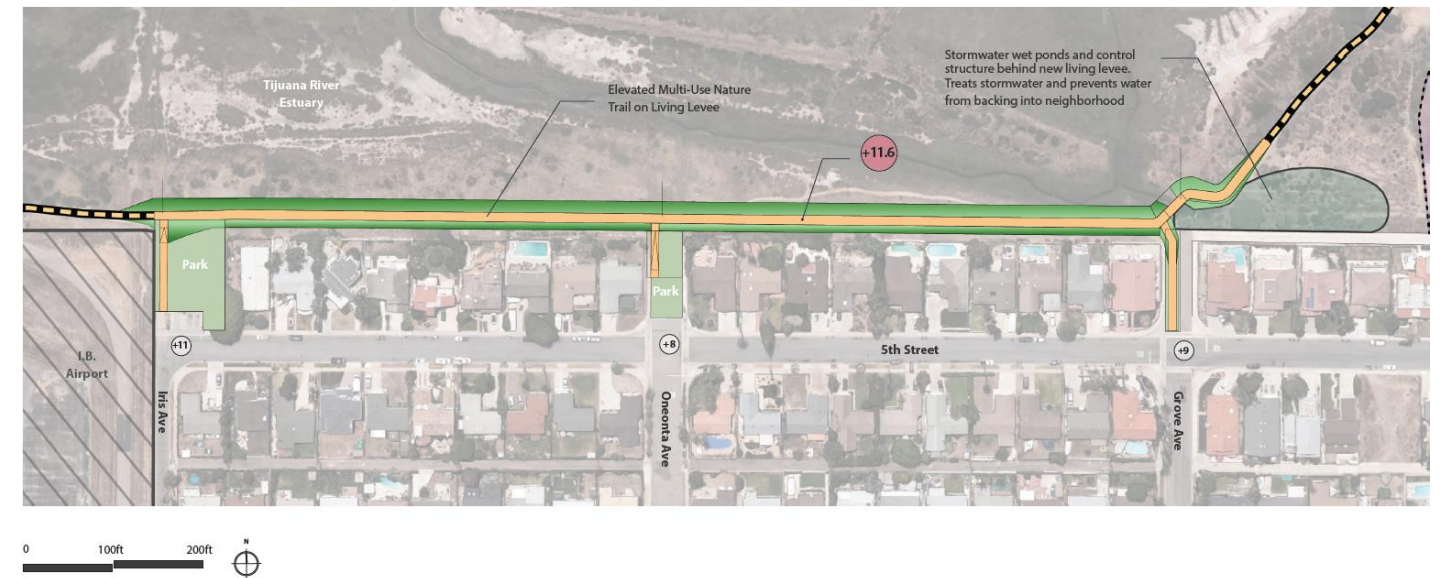
Figure 11. Plan View of Conceptual Elevated Trail and Ecotone Slope with the Street Ends of Iris Avenue and Oneonta Avenue Converted to Parks
