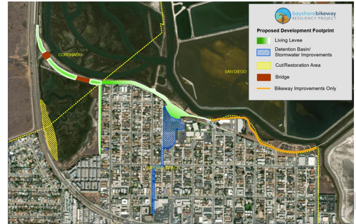
Figure 2. Bayshore Bikeway Resiliency Project Proposed Development Footprint Representing Phase 1 Adaptation for Segment 1
