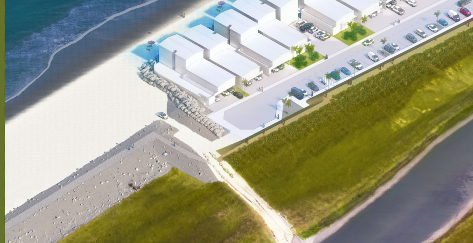
Figure 23. Cobble Berm + Ecotone Slope
