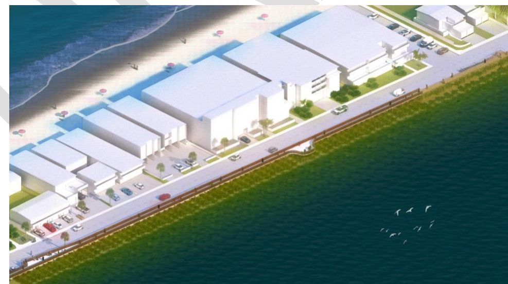
Figure 8. Conceptual Rendering of Boardwalk and Flood Wall that Transitions to Ecotone Slope Path along Seacoast Drive
