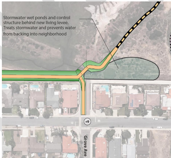
Figure 12. Plan View for Conceptual Stormwater Wet Ponds and Control Structure
